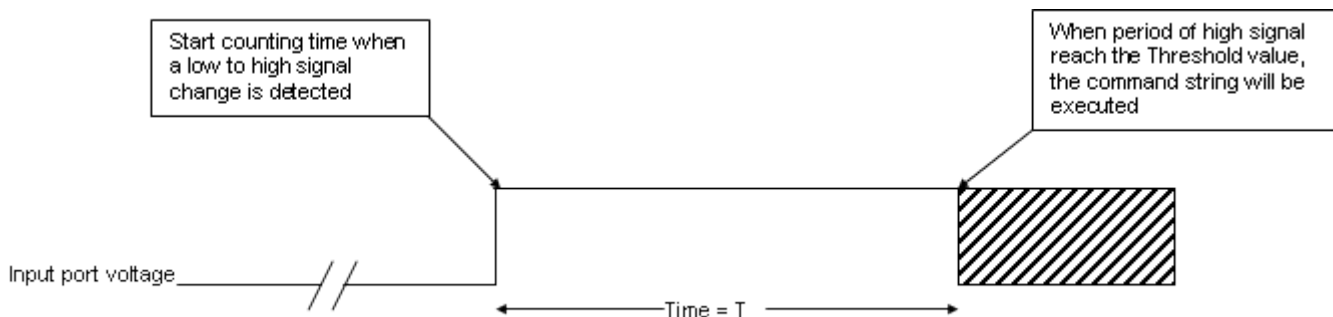
Figure 21.4.1: When T=1second the Command String #5 will be executed
